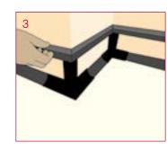
Install Capping or Diminishing Strip overlapping the Floormitres at the external and internal points.
